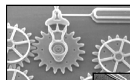
MicroElectroMechanical (MEMS) devices 10 -100 \mu\text{m} wide
